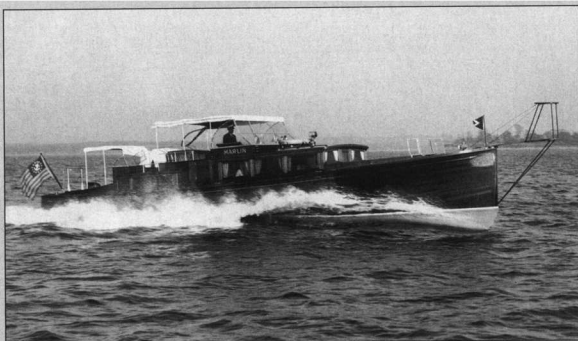
Marlin , built in 1930 to a design by Walter McInnis, is an example of a refined yacht based on the fast rumrunners of the 1920s that achieved good performance with limited power.
