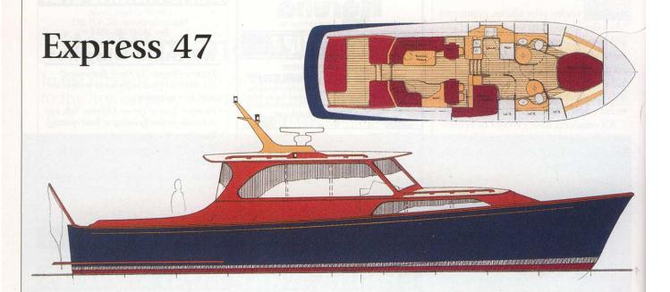
This handsome cruiser was designed by Gabriola Island naval architect Tad Roberts for Philbrooks Boatyard in Sidney, which is currently negotiating with a buyer. She's based on Roberts' successful lobster boat hull designs—seaworthy, semi-displacement hulls that make efficient coastal cruising vachts or weekending "picnic boats."
