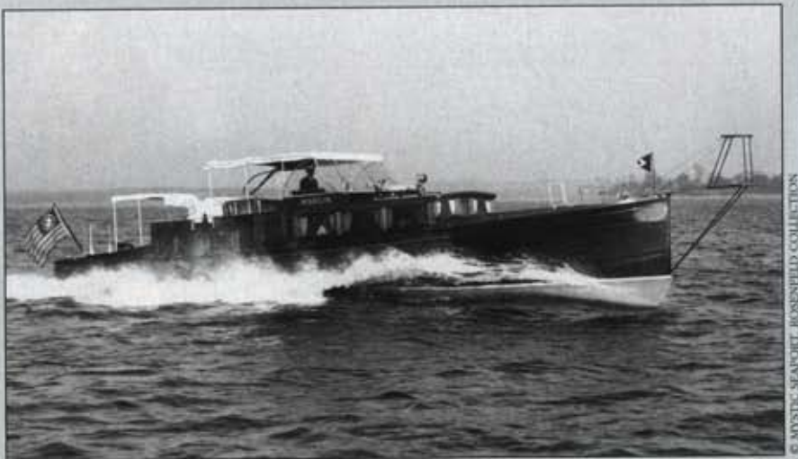
Marlin , built in 1930 to a design by Walter McInnis, is an example of a refined yacht based on the fast runrunners of the 1920s that achieved good performance with limited power.
