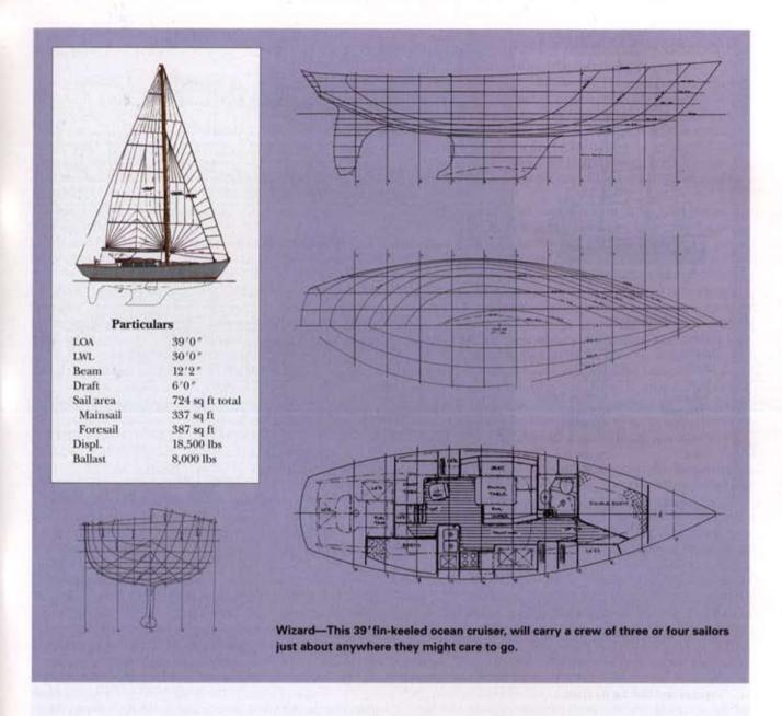
rounded sections are important amidships, where straighter sections make hulls look slab-sided. This roundness is also important aft; again, this is a modern design so the quarters are fuller (beamier) than earlier designs. The fuller quarters mean he picks up power (stability) as he heels. If this is carried too far, the boat trims down by the bow as he heels—a major contributor to balance instability and steering problems.
