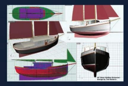
My 42' Halibut Motorsailer designs are modeled on the heavy displacement commercial fishing "schooners" that have chased halibut in the North Pacific for the last 100 years or so. The Halibut Schooner 42 has a low rig and bowsprit; Halibut Ketch 42 is ketch-riggged with a flying bridge. The hulls are multi-chine full keel with a round stern. Steel or wood construction.
